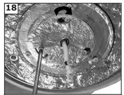
Install light plate by twisting plate with key hole slots into place. Replace screw removed and tighten the 3 screws securely.
